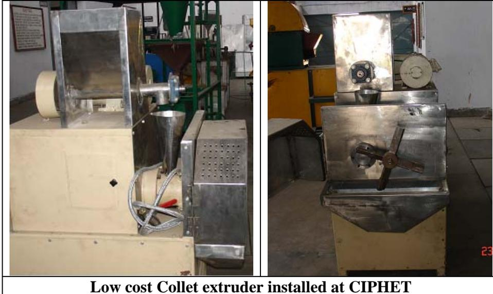
**Low cost Collet extruder installed at CIPHET**
